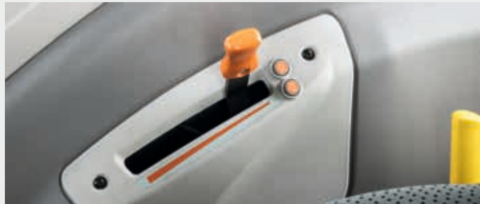
Electronic hand throttle with two engine memory speeds.
