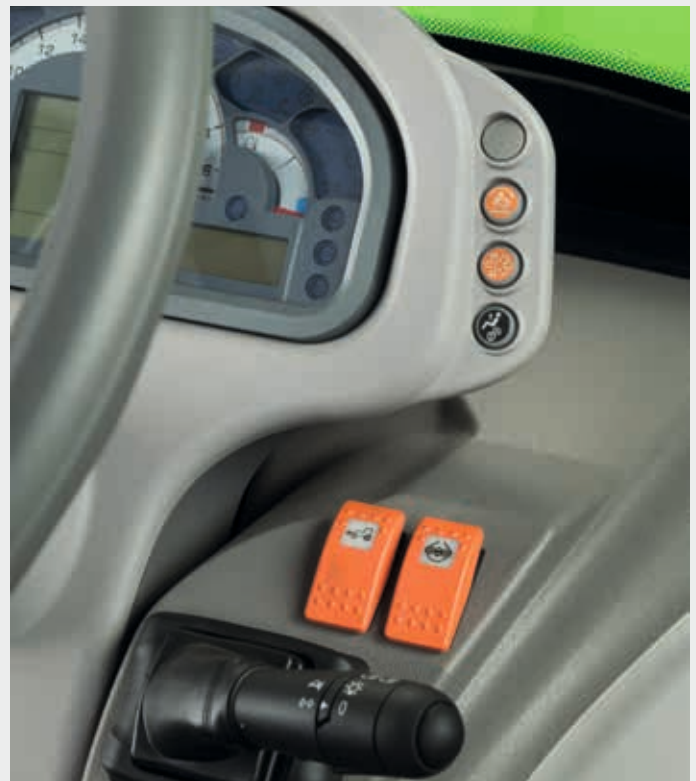
↑ Electro-hydraulic engagement for 4WD and Diff. Lock.
