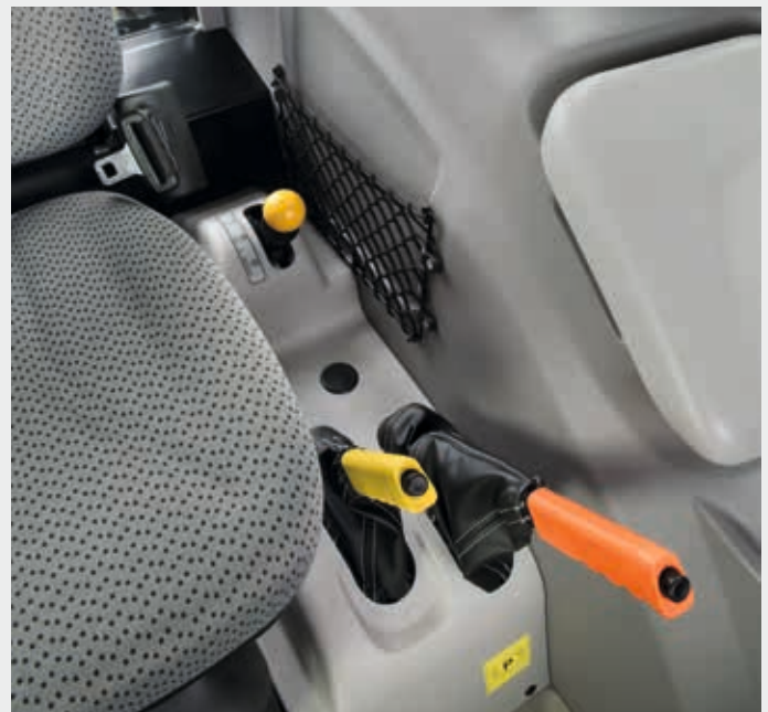
Up to 3 PTO speeds with mechanical engagement.
