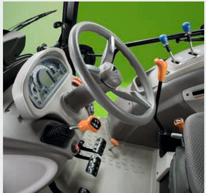
Five speed gearbox with mechanical shuttle on dashboard.
