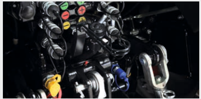
Up to 3 rear spool valves with flow regulator and free hydraulic oil return.
