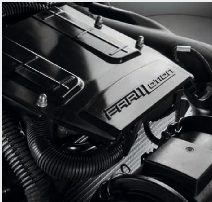
Stage V compliant FARMotion 35 engines with Common Rail injection and power outputs up to 102 HP.
